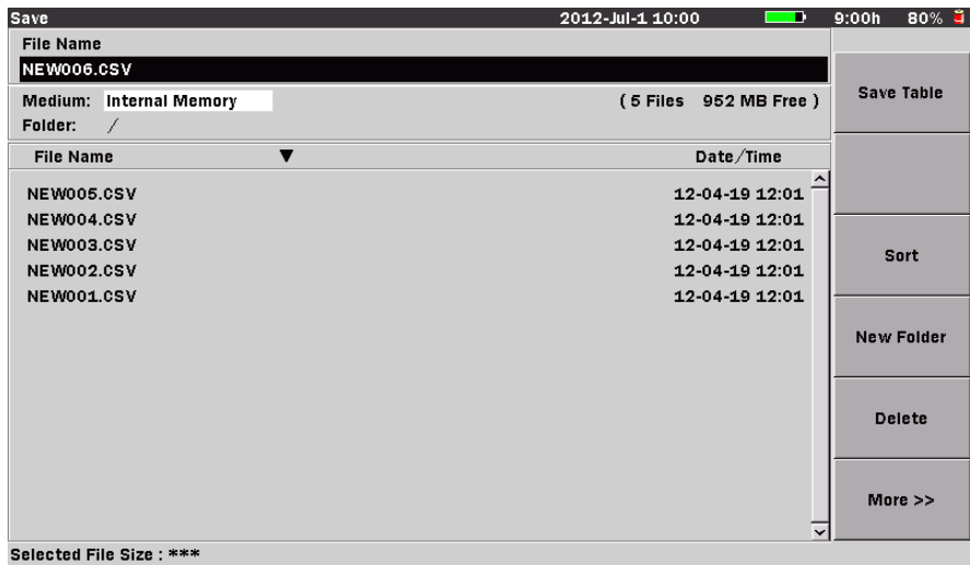
Figure 8-13: Save screen – Loss Test Set mode
